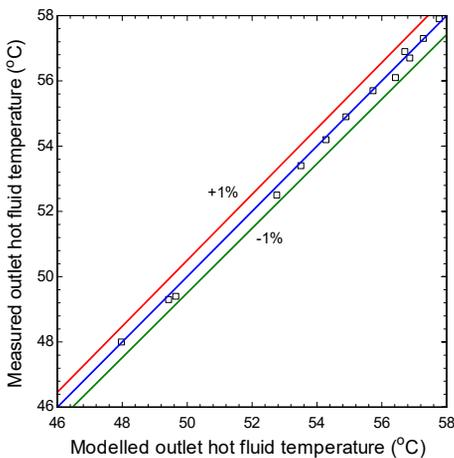
**Fig. 5: Experimental vs. theoretical outlet hot fluid temperature**
