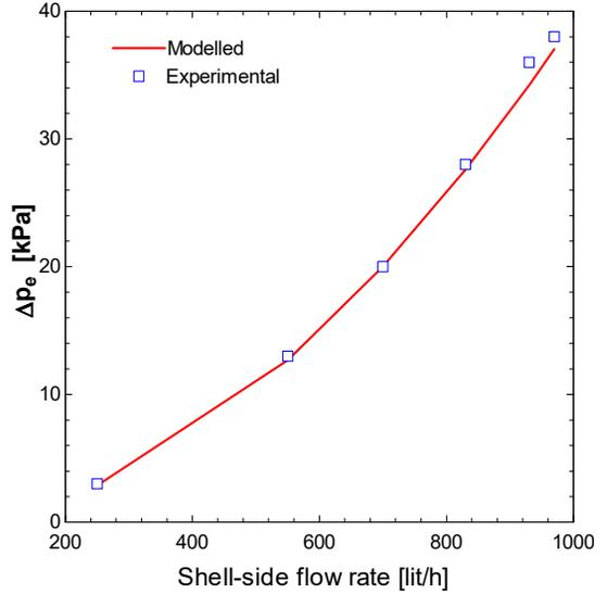
**Fig. 6: Shell-side pressure drop**
