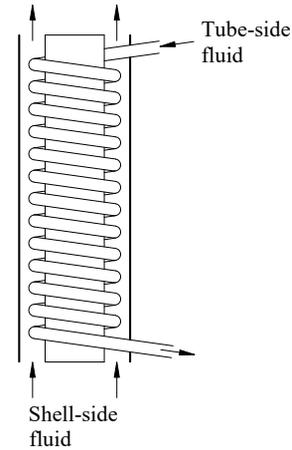
**Fig. 1: Helical coil heat exchanger**
