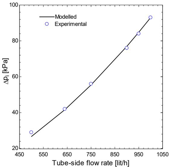
**Fig. 7: Tube-side pressure drop**
